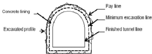
TYPICAL CROSS SECTION OF TUNNEL 4.50 m dia.
